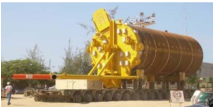
Figure 1 Example of suction anchor pile to mitigate pipeline walking (Jayson et al, 2008)
