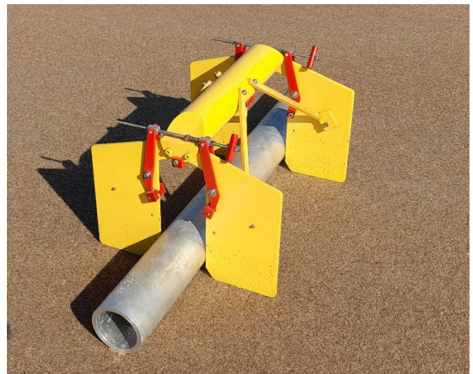
Figure 15 VEPLA configuration shown over a mock-up pipeline prior to penetration
